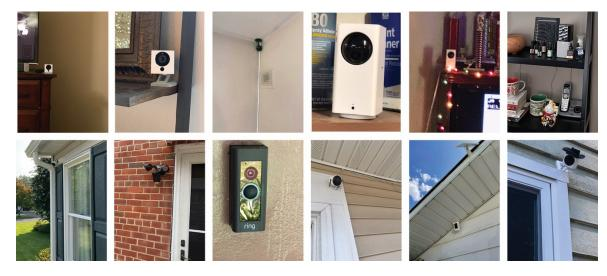
Figure 2: Examples of participants' indoor, outdoor, and doorbell smart cameras. The top row of images depicts various indoor camera placements, and the bottom row depicts outdoor camera placements. Notable images include a camera mounted upside down on the indoor ceiling, a camera placed among other domestic objects on a bookshelf, and an outdoor camera adorned with a small, decorative cowboy hat.
